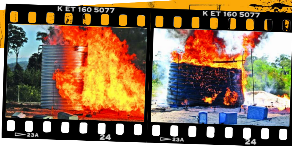
^ The plastic tanks collapsed when exposed to continuous flame immersion for a period of 30 minutes.
